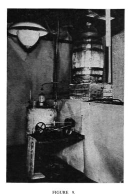
Apparatus Used in Continuous Feeding Investigation on Anaerobic Fermentation of Cellulose, Tank A.
